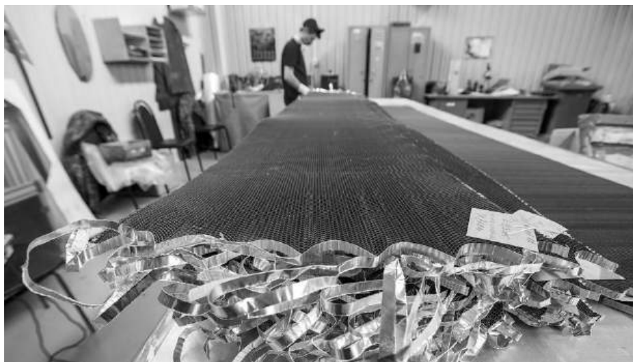
Figure 1.7 – Cell block after stretching
