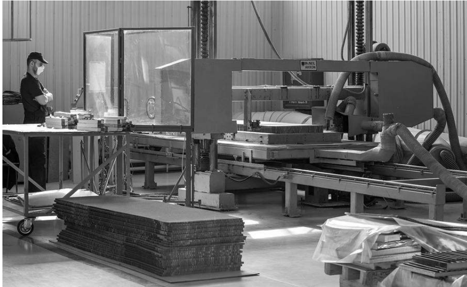
Figure 2.5 – Cutting of honeycomb packages from polymer paper
