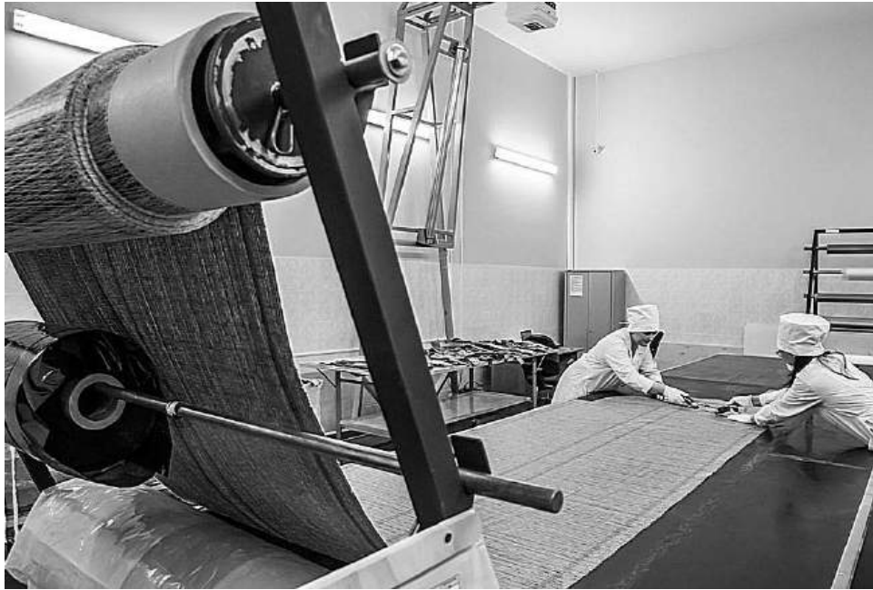
Figure 2.7 – Cutting the fabric using a laser projector
