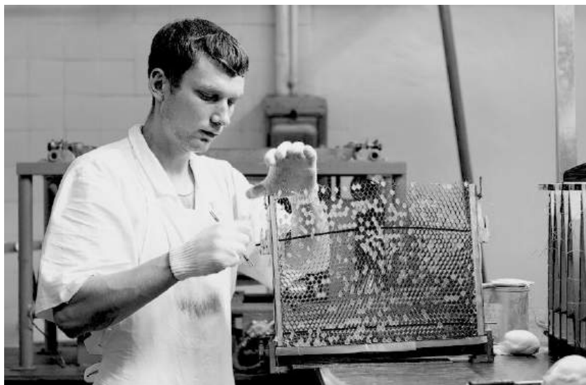
Figure 1.14 – Fixing the honeycomb filler in the layout of the frame of the honeycomb structure
