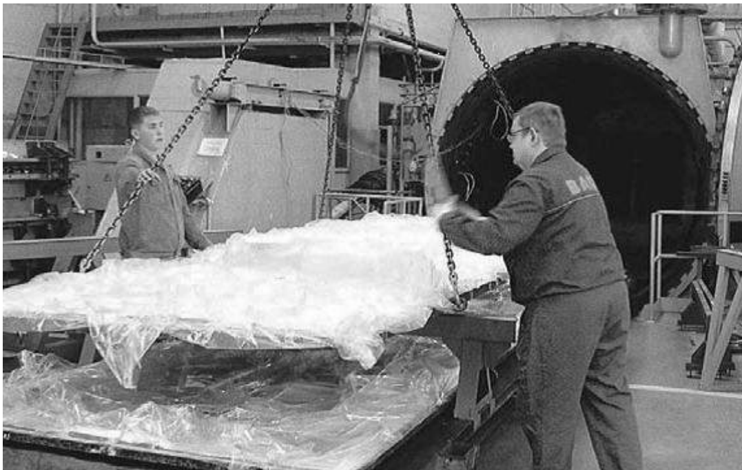
Figure 2.11 – Load into the autoclave of the sticker forms
