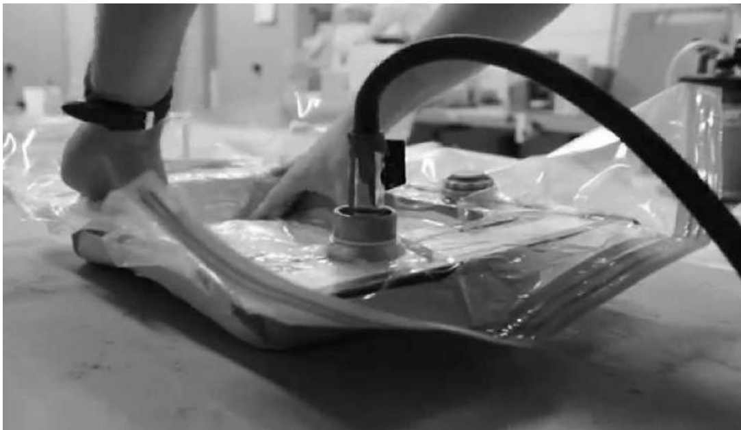
Figure 2.14 – Vacuum bag for forming the shell of the compartment
