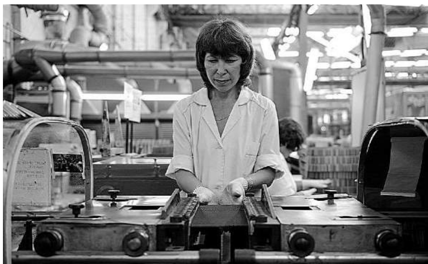
Figure 1.8 – Stretching the honeycomb block of the tail unit of the blade
