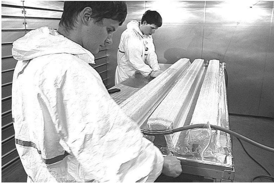
Figure 2.10 – Packing the sticker into a vacuum bag
